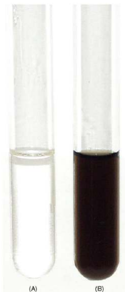
Fig. 1. Streptomyces antibioticus tyrosinase. (A) The exocellular enzyme was purified by a combination of PEG-8000/phosphate aqueous two-phase system plus ammonium sulphate fractionation (0–60%). (B) The exocellular tyrosinase was only purified using ammonium sulphate fractionation (0–60%) as described in literature for Streptomyces glaucescens [2].
