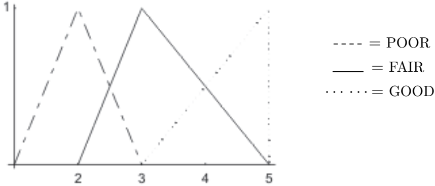
Fig. 2.3: Fuzzy values of the CURRENT CONDITION OF THE PIERS of the highway bridges
