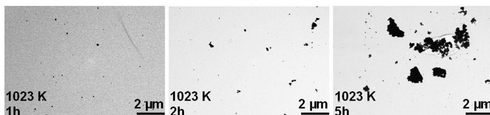
Figure 3.34. TEM micrographs for a 1 % Tm, 0.5 % Ho, 1 % Yb:KLuW nanocrystals after isothermal annealing at 1023 K.
