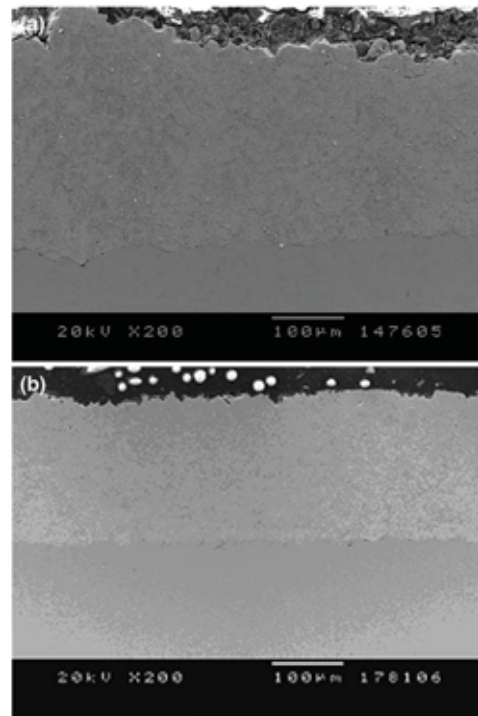
Fig. 5 (a) SEM structure of A-625 after E-C test and (b) SEM structure of B-625 after E-C test
