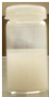
Figure 6.2. Photograph of the Eu^{3+}:(1\%)Bi^{3+} -CPechl nanopowder after its dispersion in THF solvent by using the ultrasound bath technique.
