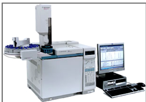
Figure 3.3: Gas chromatograph coupled to a electron capture detector (GC-ECD), with automatic injector.
